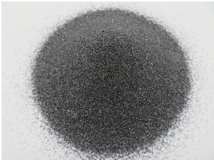
It is black and features brittle and sharp, certain capacity of heat-transmission and electricity-transmission. Its Knoop hardness is 3100-3280kg/mm<sup>2</sup>. It can be used for making bonded and coated abrasives, which are suitable for grinding metal and non-metal materials with lower tensile strength, such as gray cast iron, brass, aluminium, stone, leather, rubber, paint, wood, etc. Besides, it can be also used for refractories.
